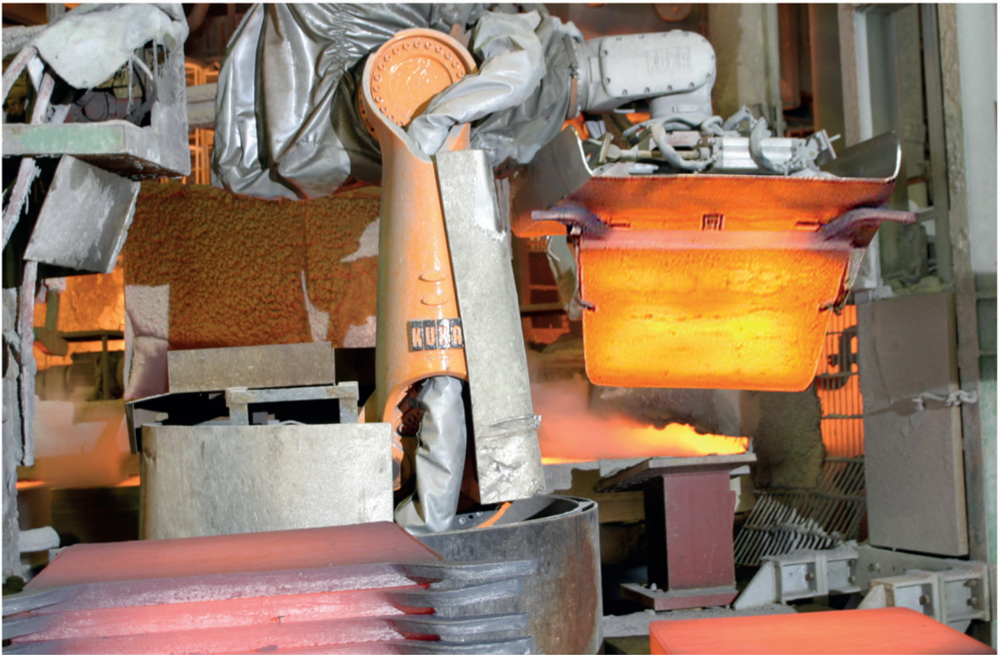
Handling-Robots for cast copper anodes: Temperature at reception 800°C
