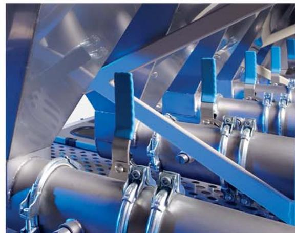
After a longer period of time (approx. 300 to 400 running hours) the fine mashed conveyor belt is cleaned to prevent clogging. A separate cleaning cycle is started by pressing water through the screen belt using two lines of high-pressure nozzles. Subsequent line of nozzles blow compressed air through the screen belt. Water separator and sound absorber are parts of the cleaning chamber.
