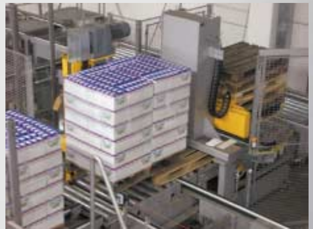
Unstacking of 2 x 1/2 pallets (Düsseldorfer) and stacking of Euro pallets up to 20 units.
