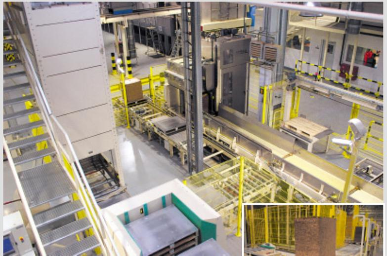
Parallel to the cutting device special stainless-steel pallets are supplied.
