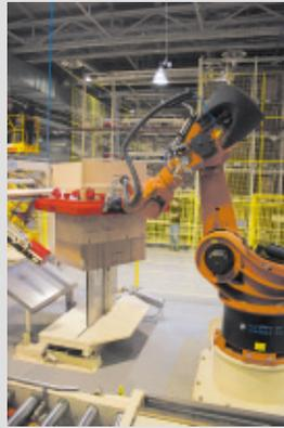
After automatic dismantling: Cartons are picked by robot and supplied to the folder.
