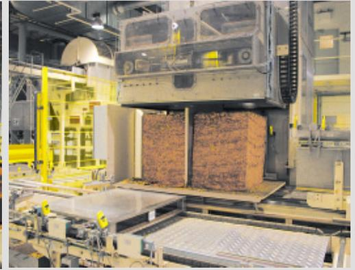
Cutting device (divider): It centers the bale and exactly divides it into 50/50%.
