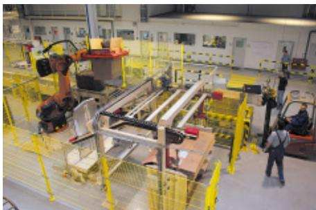
The dismantling mainly consists of five-axis-robot, a carton folding unit and a carton stacking device.
