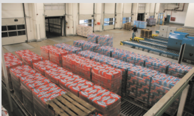
Individual consignment goods ready for delivery, shown as a flow storage with separation mechanics at the appropriate end of the lane
