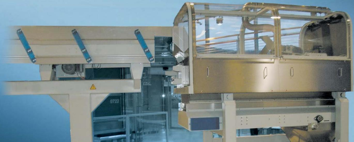
The Tobacco String Remover **TSR** is developed to remove long-fibred foreign bodies like strings or feathers from leaf tobacco and/or various blends. Cleaning of the tobacco is effected by 6/8 picking rollers lined with a food-proof “scraping” belt fitted with stainless steel pins. Foreign bodies are caught and held in the needles of the scraping belt without any damaging effect on the tobacco.
